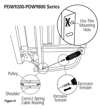
**TIP:** If door does not open easily or falls too quickly, check the spring cable routing. Check that the cable is properly aligned on the pulley (as shown).
